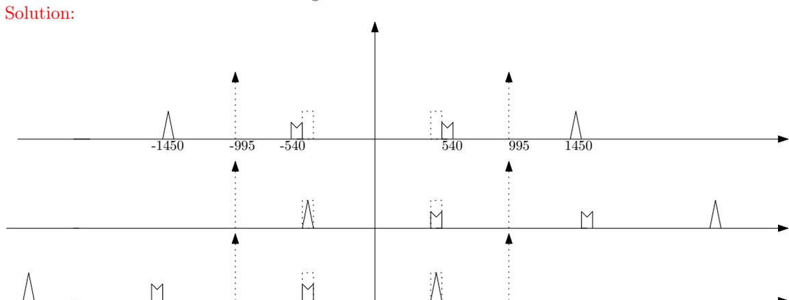
Clearly, there would be corruption here because one copy of each signal lands in the IF band. To prevent this, we must eliminate the image station prior to downconversion to IF. The problem of overlapping spectra after up and down conversion is more general and the potential for a problem like this should ALWAYS be kept in mind when translating frequencies.
